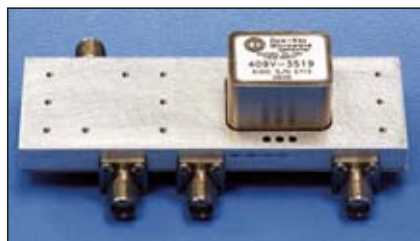
Fig. 1 The 409 switch mounted in a PCB fixture.
